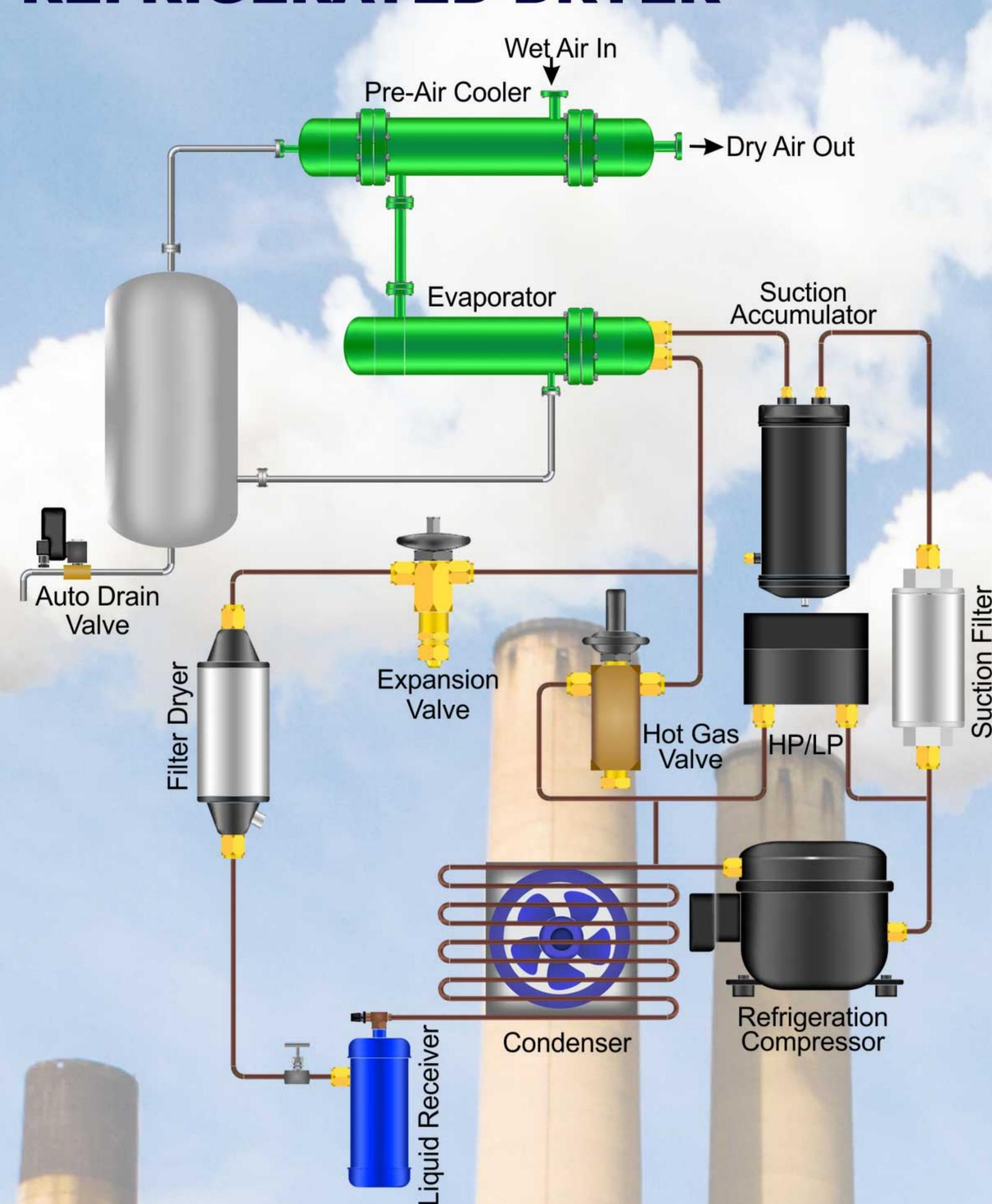
Our refrigerated type of air dryer is based on principle of the removal of moisture by cooling air to certain present temperature. As there is no concept of cooling of a body. Cooling refers to the removal of the heat from a body. The air to be dried is subjected to the pre cooler unit and evaporator unit. After this air get condensed and this moist air is passed through a moisture separator where moisture is drained out by centrifugal action of air
