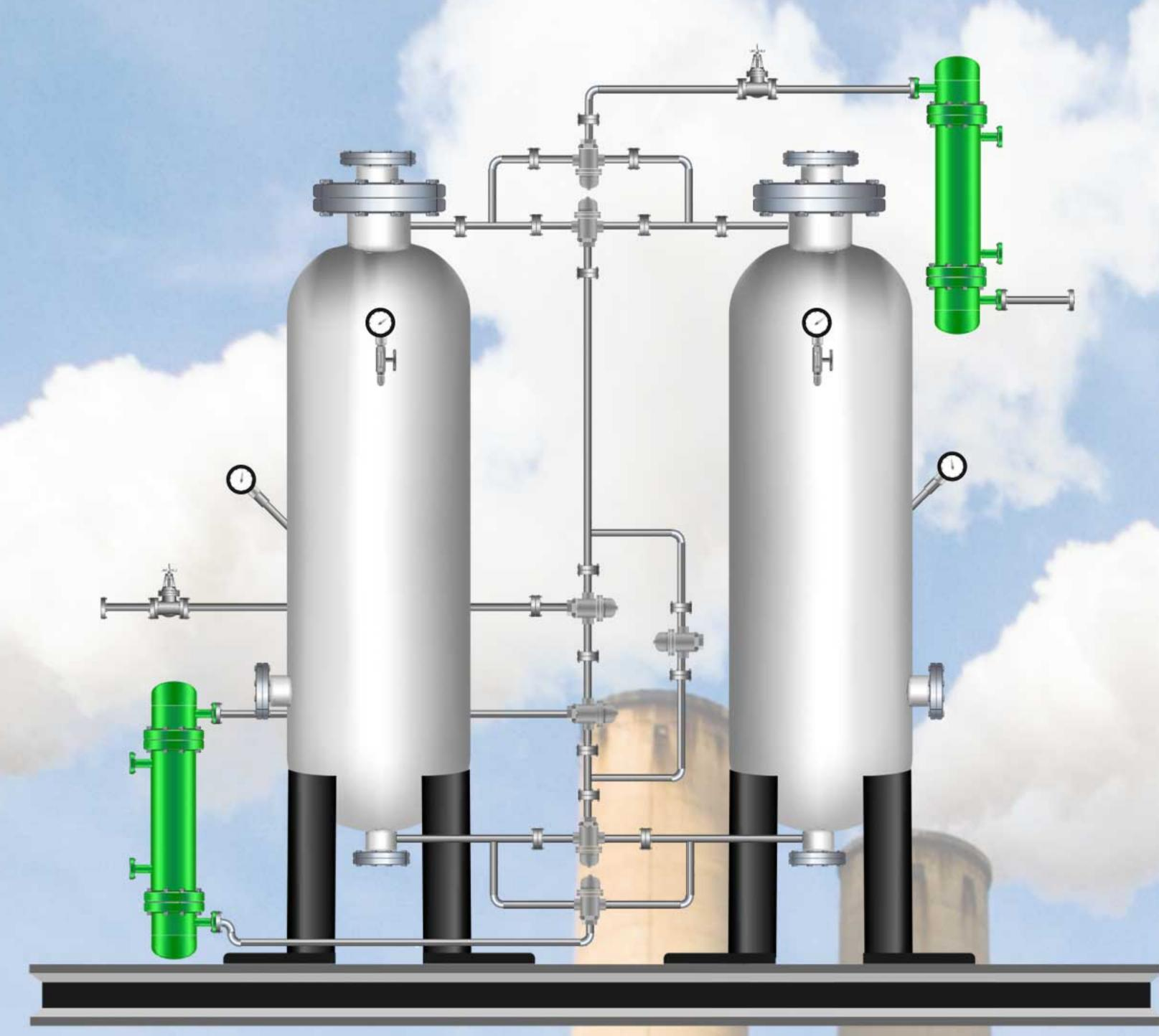
An air compressor generates heat. This heat is normally lost when the compressed air stream is cooled after the compressor. The quest of an HOC dryer is to utilize this waste heat for desiccant bed regeneration and thereby eliminate the use of an external heater. The basic idea is to directly flow all or part of the hot compressed air through the regenerating desiccant bed prior to cooling and adsorption.
